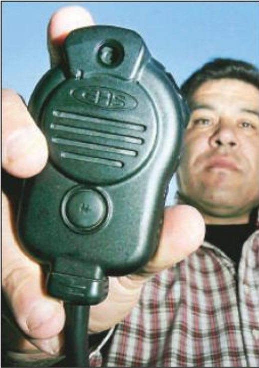
David Swanson displays the Vidmic, a device for law enforcement in which a full-color digital video and audio recorder, as well as a still photo camera, is housed in a shoulder microphone.
