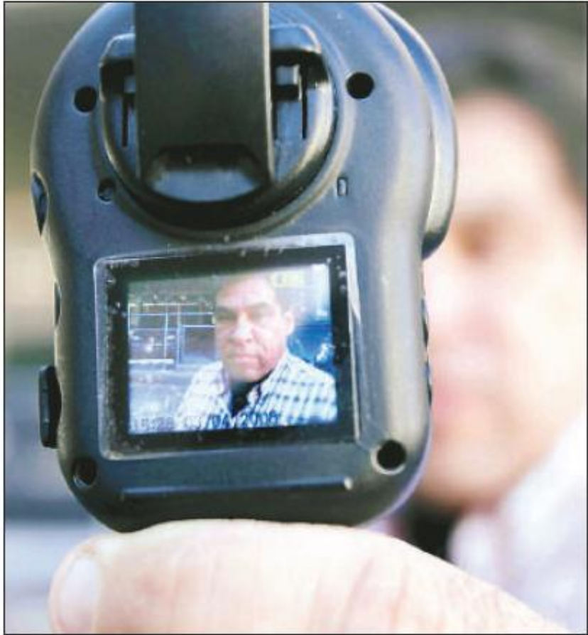
David Swanson displays the Vidmic, a device for law enforcement in which a full-color digital video and audio recorder, as well as a still photo camera, is housed in a shoulder microphone.
